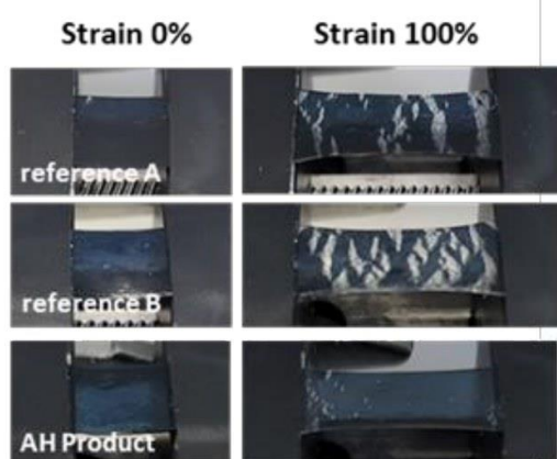
Films at 0 % and 100 % strain: references A, B vs. AH product
